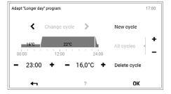
The overview of the selected day program is opened. Various adaptations can be made to the selected day program/switching cycle using **plus** (+) and **minus** (-). Press **OK** to accept the entry.
