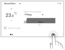
The active day program and the set room temperature can be seen on the screen. Accept the setting with **OK**.
