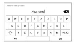
A **keypad** appears on the screen that you can use for renaming the selected week program. Press **OK** to accept the entry.
