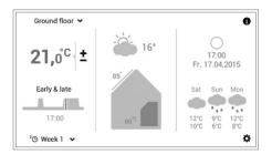
The current room temperature is displayed on the start screen and goes up or down until the desired room temperature is reached.
