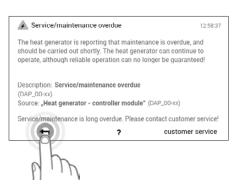
A detailed alarm message appears. The message contains detailed information about the malfunction. Use **Back** ( ) to close the alarm message view.
