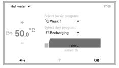
Hot water recharging is shown in the menu. Confirm the entries with **OK**.
