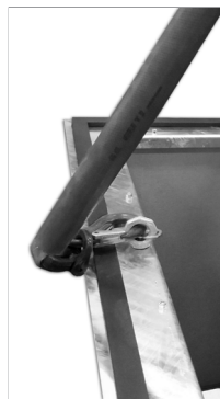
Fig. 21: Transport eye in the connection module
