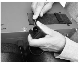
3. Change fuse. A replacement fuse (E) is available in the insert. The defective fuse can be disposed of in household waste.
