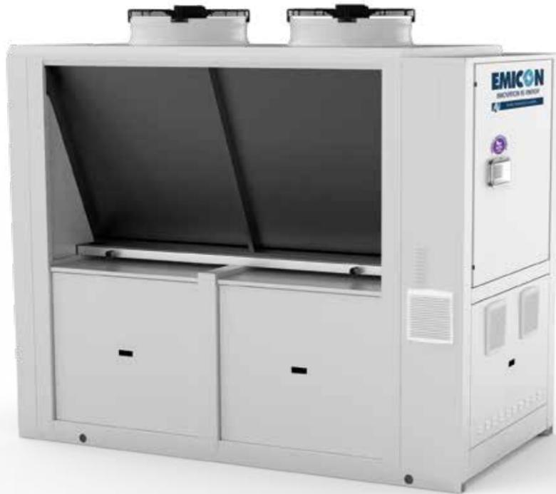
EMICON's packaged air-cooled reciprocating chillers for outdoor use with free cooling, using highly sustainable R290 refrigerant, are suitable for high temperature process cooling applications, data centres and in general where cooling is required all year round. When the outdoor ambient temperature is sufficiently low, the integral free cooling coils allow cooling without operating the compressors.
