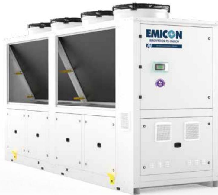
EMICON's packaged air-cooled reciprocating chillers for outdoor use, suitable for HVAC and high temperature process cooling applications. Microchannel condenser coils mean only a minimal charge of highly sustainable R290 refrigerant is required.
