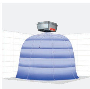
Cooling operation: The inflowing air is colder than the room air and sinks. To avoid draughts, it is injected horizontally.
