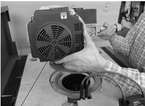
Fan and gas mixing device
